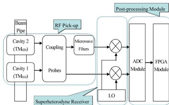
Figure 1: The schematic diagram of a single cavity.
