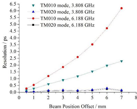
Figure 10: Resolutions vary with beam position offsets.
