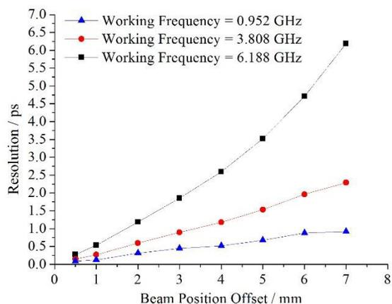
Figure 6: Resolutions vary with beam position offsets.
