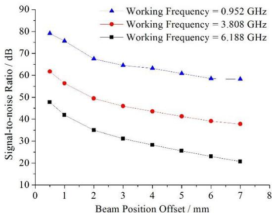
Figure 5: SNRs vary with beam position offsets.
