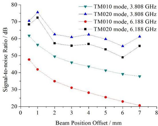
Figure 9: SNRs vary with beam position offsets.
