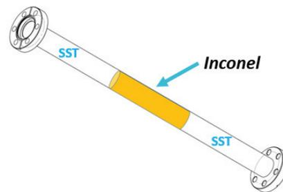
Figure 2: Quadrupole doublet chamber with Inconel segment.
