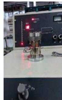
Figure 8: Flange under leak check.
