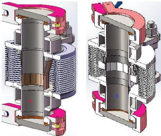
Figure 9: Two configurations of RF shielded bellows (A-outside finger; B-omega stripe).
