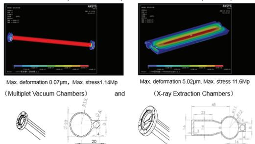
Figure 4: Multiplet chamber and X-ray extraction chamber.
