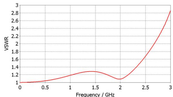
Figure 8: VSWR of the feedthrough.
