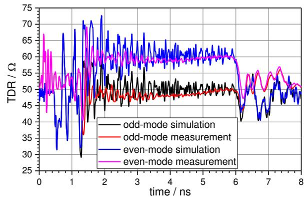
Figure 11: TDR Comparison between simulation and testing results.
